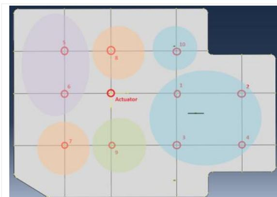
Fig. 13a: Detectability Map for a 20 mm Crack
