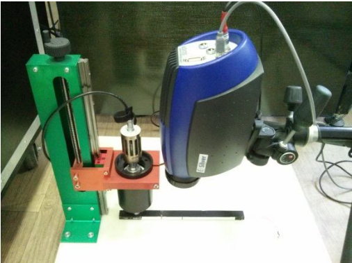
Pic. 10. Vibrothermographic test setup
