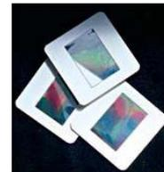
Holographic diffraction grating film [ED18]
